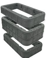
Each chamber is made from 150mm deep riser and access sections, which interlock to offer flexibility in finished chamber depth. Each section is profiled to positively interlock with the units above and below. Each access section has various entry/exit points depending on their size.
