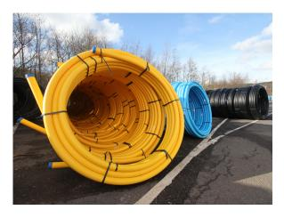
The material used to manufacture blue or black pipes at 90mm or above is generally **HPPE or PE100**. This is a stronger and denser product than PE80. The sizes range from 90mm all the way up to 1200mm if required, with **SDR** (Standard Dimensional Ratio) options to suit different pressure requirements (a high SDR denotes a lower pressure rated pipe). Coils are available up to 180mm, however lengths are available in all diameters.
