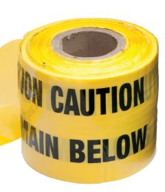
Laid half way between a pipe and the surface within a trench, Underground Warning Tape is printed with a warning text to warn future excavators of the presence of a pipe below.
